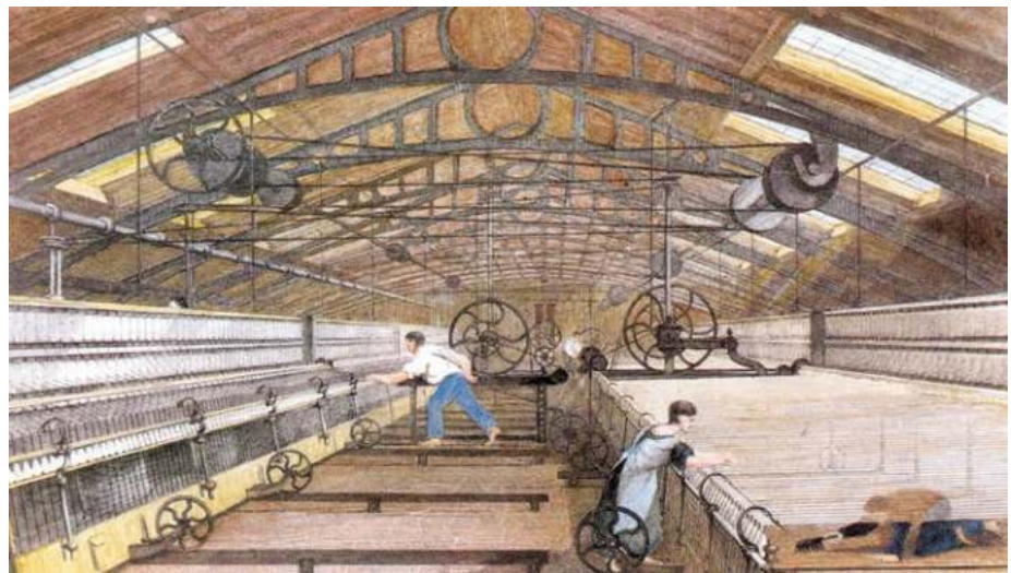
Fig. 7 – A spinning factory in 1830. You can see how giant wheels moved by steam power could set in motion hundreds of spindles to manufacture thread.
